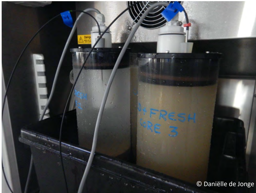
Figure 11. Set-up of the multi-stressor incubation experiment during a SCOC measurement interval. Sediment in cores, sealed at the bottom, are placed in buckets of water, and located in cooled incubators. The sealing lid carries the stirrer bar (white) and FireSting oxygen optodes (blue label). After the SCOC interval, the lid including stirrer and optode were removed, and an air stone was replaced to oxygenate the open core. Note that this image was taken shortly after sampling i.e. before the 1-week equilibration period, and the overlying water in some cores were somewhat cloudy.
